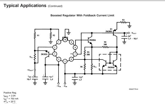
$\begin{array}{l} \mbox{Positive Reg.} \\ I_{MAX} = 2.0A \\ I_{SC}^+ = 750 \mbox{ mA} \\ @T_A = 25'C \\ +V_{IN} = +25V \\ \mbox{Negative Reg.} \\ I_{MAX} = 2.0A \\ I_{SC} = 750 \mbox{ mA} \\ @T_A = 25'C \\ -V_{IN} = -25V \\ \end{array}$
