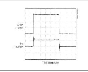
Figure 13. Shutdown Enable/Disable Supply Current
