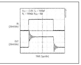
Figure 9. Small-Signal Transient Response with Excessive Capacitive Load
