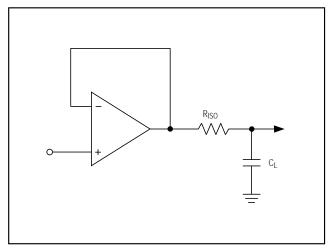
Figure 11. Capacitive-Load-Driving Circuit
