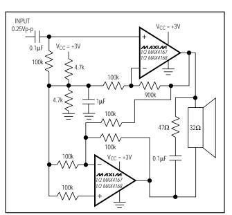
Figure 3. Dual MAX4167/MAX4168 Bridge Amplifier for 200mW at 3V
