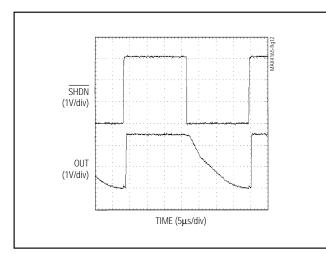
Figure 12. Shutdown Output Voltage Enable/Disable
