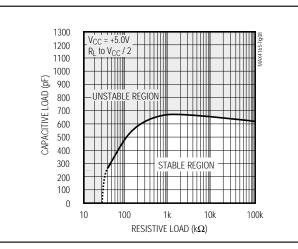
Figure 8. Capacitive Load Stability
