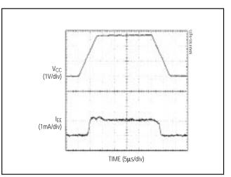
Figure 15. Power-Up/Down Supply Current
