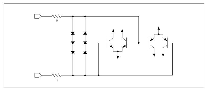
Figure 6. Input Protection Circuit
