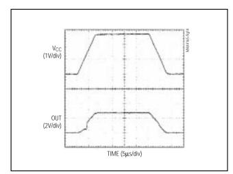
Figure 14. Power-Up/Down Output Voltage
