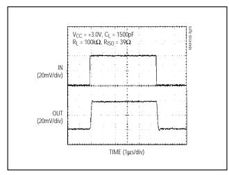
Figure 10. Small-Signal Transient Response with Excessive Capacitive Load with Isolation Resistor
