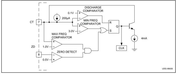
Figure 2. UC3872 oscillator section.
