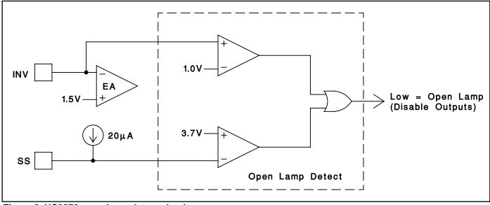
Figure 3. UC3872 open lamp detect circuitry.
