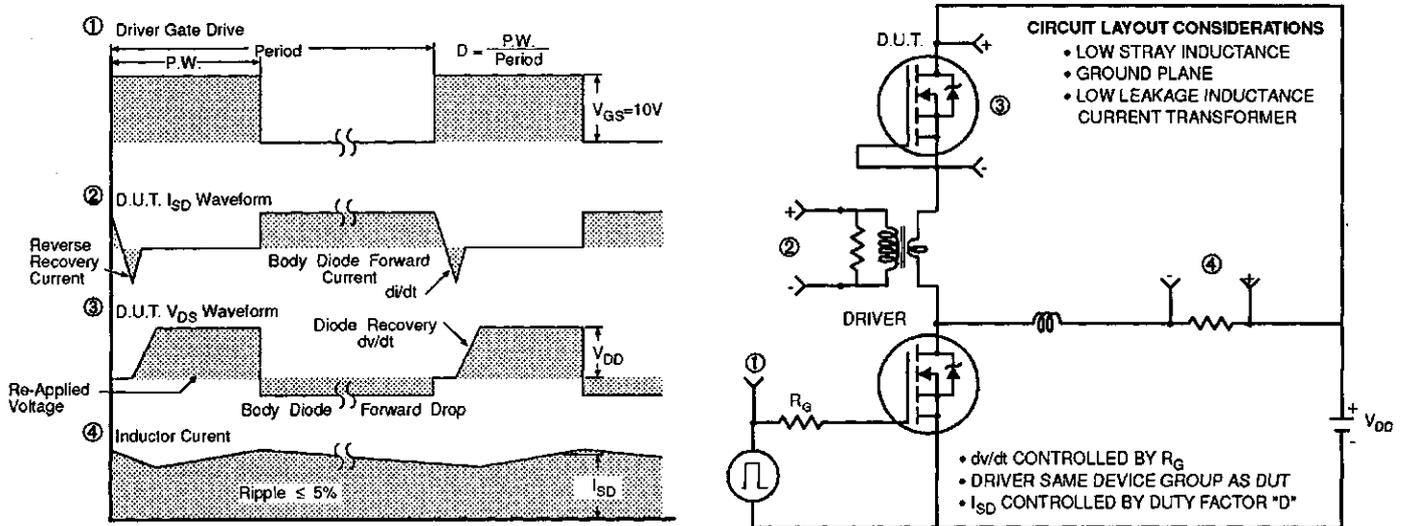
**Fig 14. Peak Diode Recovery  $dv/dt$  Test Circuit**
