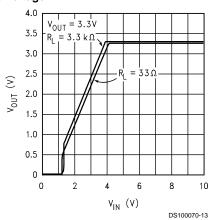
**Output Voltage** vs Input Voltage
