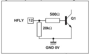
The duty cycle is adjustable through I<sup>2</sup>C from 30 % to 65 %. For a safe start-up operation, the initial duty cycle (after power-on reset) is 65% in order to avoid having too long a conduction period of the horizontal scanning transistor.
