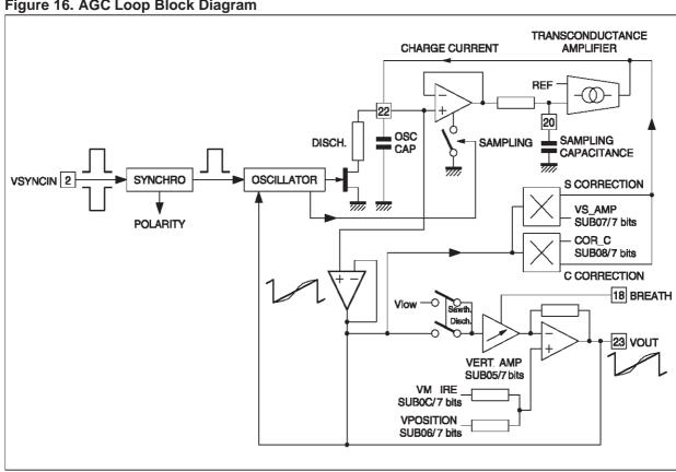
Figure 16. AGC Loop Block Diagram
