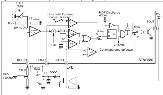
Figure 18. DC/DC Converter (represented: Step-Up configuration)
