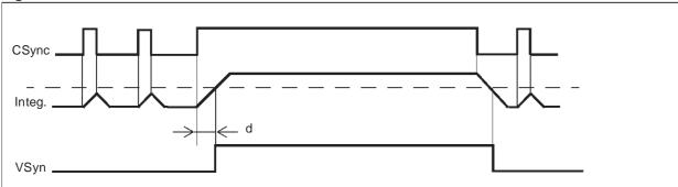
The last feature performed is the removal of these equalization pulses which fall in the middle of a line, to avoid parasitic pulses on the phase comparator (which would be disturbed by missing or ex-
