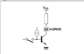
This output stage is intended for "reverse" base control, where setting the output NPN in off-state will control the power scanning transistor in off-state.
