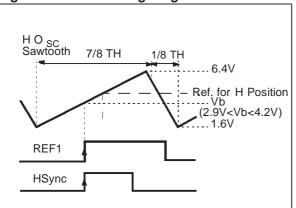
Phase REF1 is obtained by comparison between the sawtooth and a DC voltage adjustable between 2.9 V and 4.2 V.
