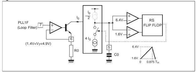
The VCO uses an external RC network. It delivers a linear sawtooth obtained by the charge and the discharge of the capacitor, with a current proportional to the current in the resistor. The typical thresholds of the sawtooth are 1.6 V and 6.4 V.
