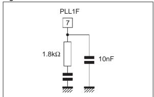
The PLL1 is internally inhibited during extracted vertical sync (if any) to avoid taking in account missing pulses or wrong pulses on phase comparator. Inhibition is obtained by stopping high and low signals at the input of the charge pump block (see Figure 8 on page 25).
