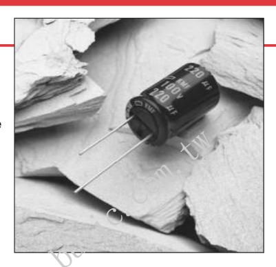
The KMF series capacitors are designed for low impedances at high frequencies with the case sizes of the KME general purpose capacitors. These capacitors will operate over a wide temperature range,  $-55^{\circ}$ C to  $+105^{\circ}$ C, with a load life of between 2,000 and 5,000 hours with the rated ripple current applied, depending on the case size.
