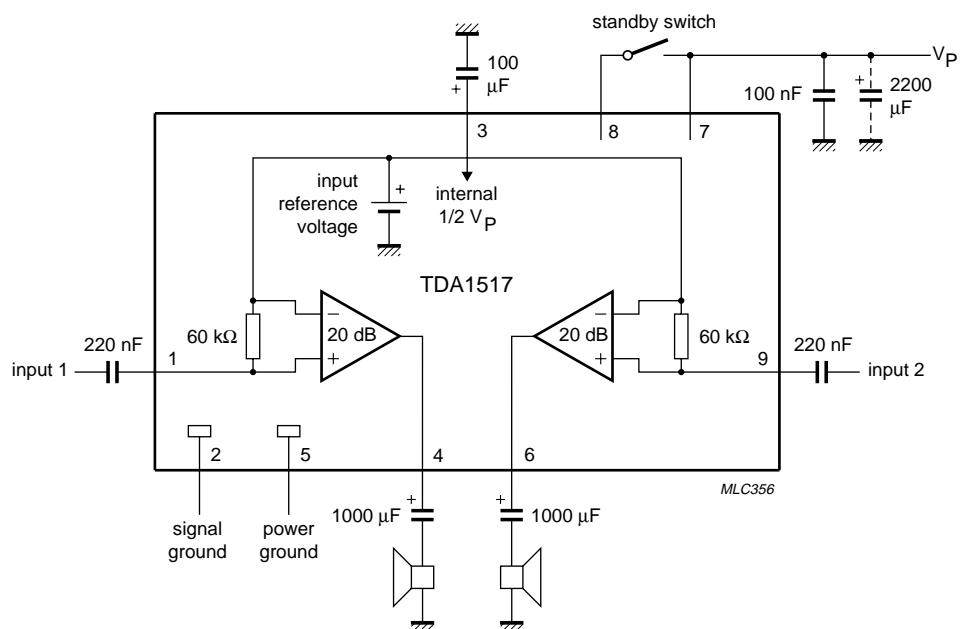
Fig.6 Application circuit diagram.
