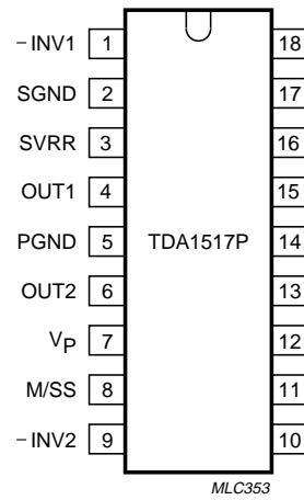
Pins 10 to 18 should be connected to GND or floating.
