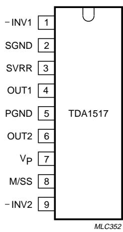
Fig.2 Pin configuration for SOT110-1.
