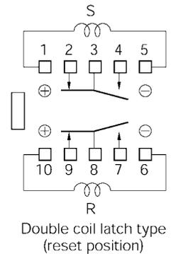
S : Coil polarity of set (operate)
