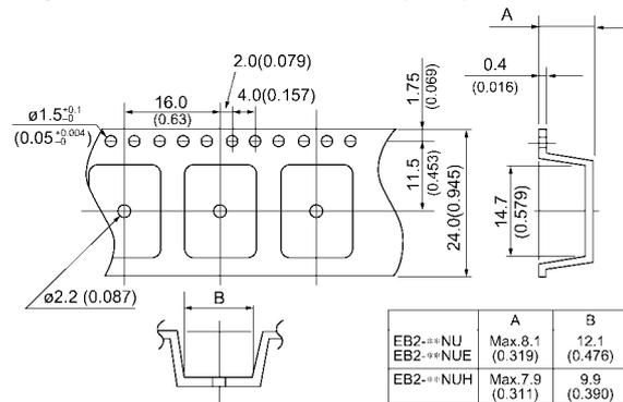
**Relay orientation mark and tape carrying direction.**
